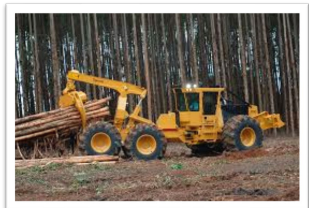
Courtesy of Caterpillar a wheeled skidder with the arch grapple transporting logs
