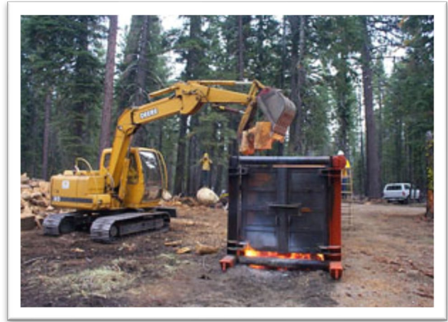
Courtesy of U.S. Forest Service San Dimas Experiment Station, Air Curtain Burner
