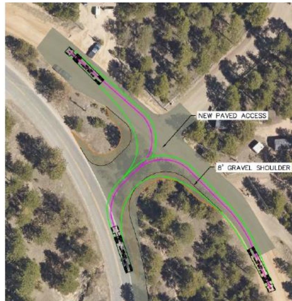
New Intersection Alignment SH 72 and Gross Dam Road
