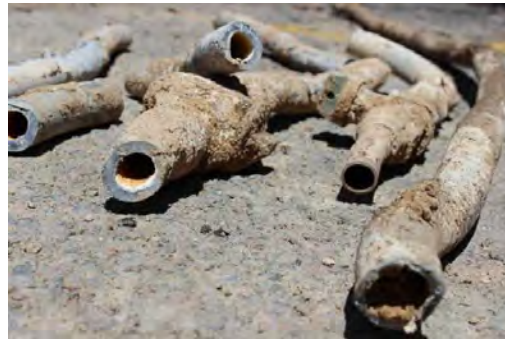
Pieces of lead service lines installed by builders decades ago. Denver Water is replacing lead service lines with new, lead-free copper lines at no direct charge to the customer.
