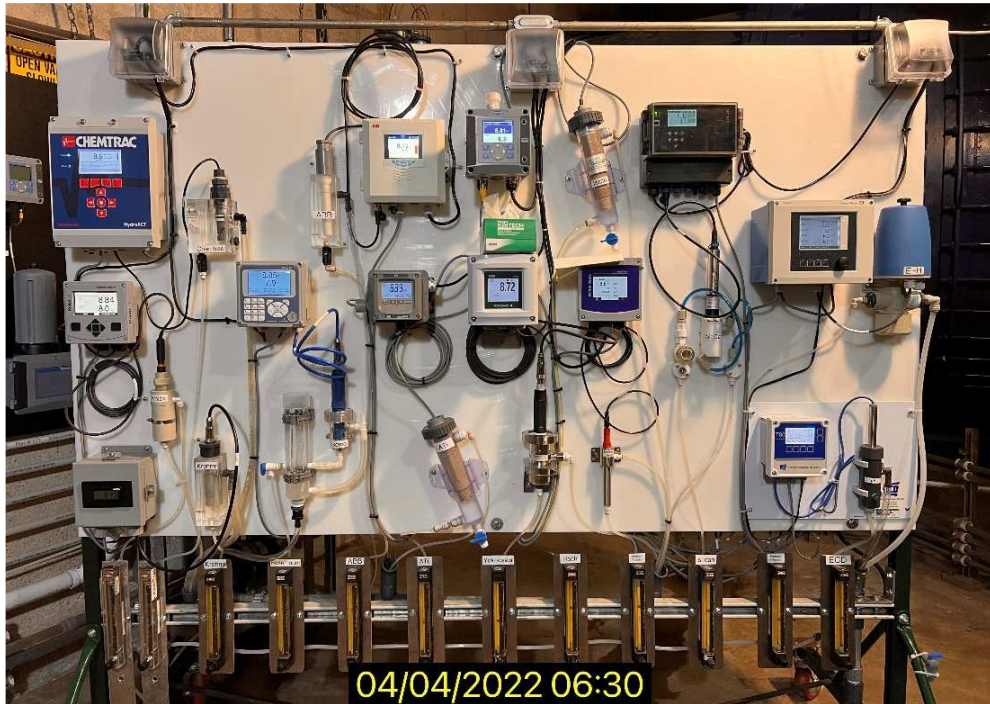
Figure 2. Photo of the pH skid used throughout the duration of the study.
